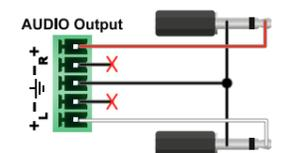
For more information about audio cable wiring see the user's manual of the device or the Audio Cable Wiring Guide on our website [www.lightware.com](http://www.lightware.com).
