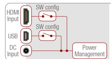
If the power adaptor is connected, it will supply the device independently from the HDMI/USB ports. If the adaptor is disconnected from the DC input connector the device tries to use a different power source (HDMI or USB) if it is enabled and connected. (If the adaptor is unplugged from the AC socket but the DC plug is still connected, the device will be switched off and cannot be changed to another power source. Unplug the DC cable from the device to be powered by USB or HDMI.)
