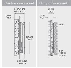
▲ Complies with U.S. ADA regulations for installed depth under 4"
